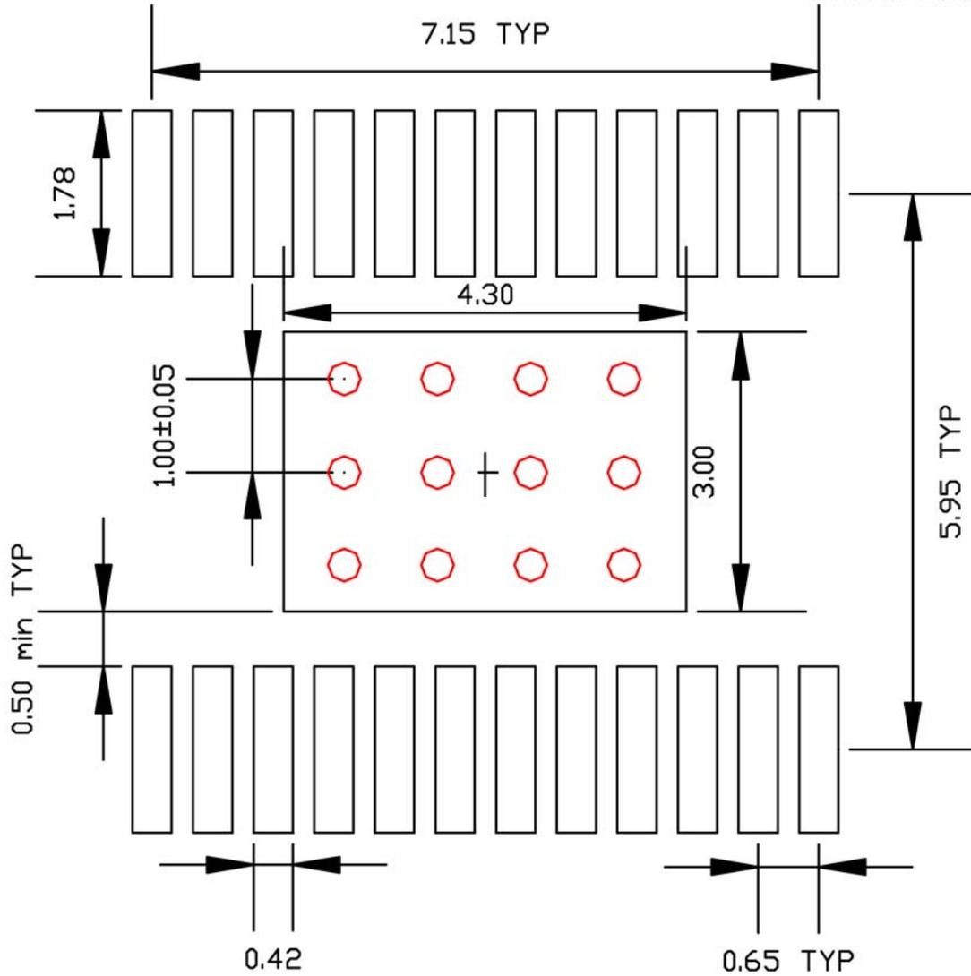
Red circle indicates Thermal Via. Size should be .300mm - .350mm in diameter, and it should be connected to GND plane for maximum thermal performance.
