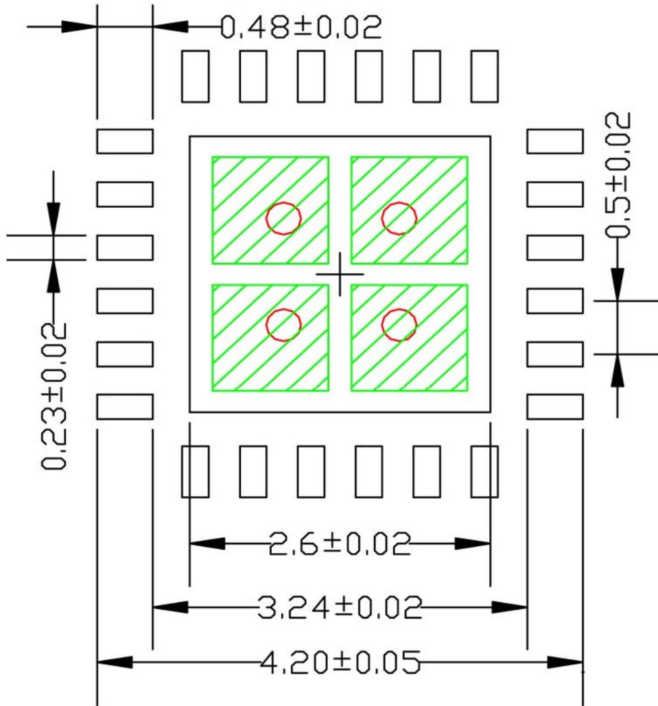
**Red circle** indicates Thermal Via. Size should be .300mm - .350mm in diameter, 1.00mm pitch, and it should be connected to GND plane for maximum thermal performance.
