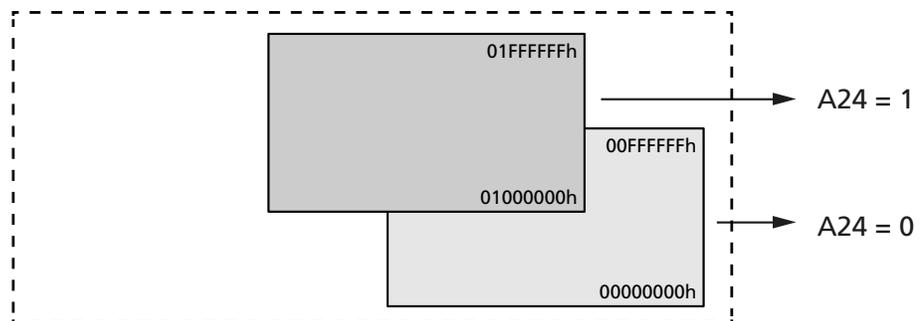
The PROGRAM and ERASE operations act upon the 128Mb segment selected in the extended address register. The BULK ERASE operation erases each 256Mb die.
