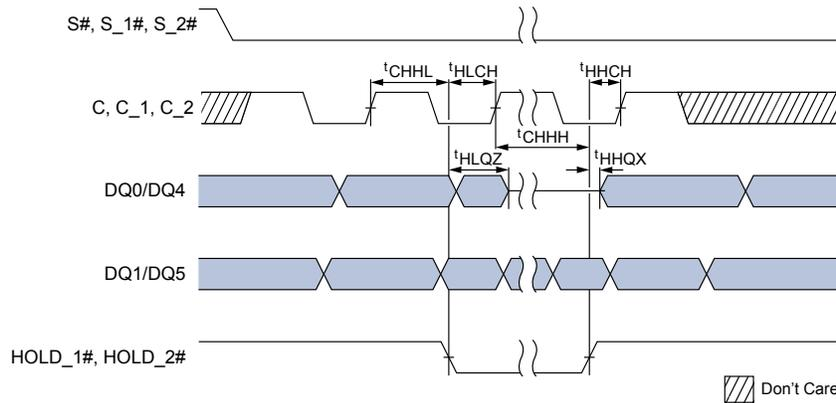
**Figure 52: Output Timing**
