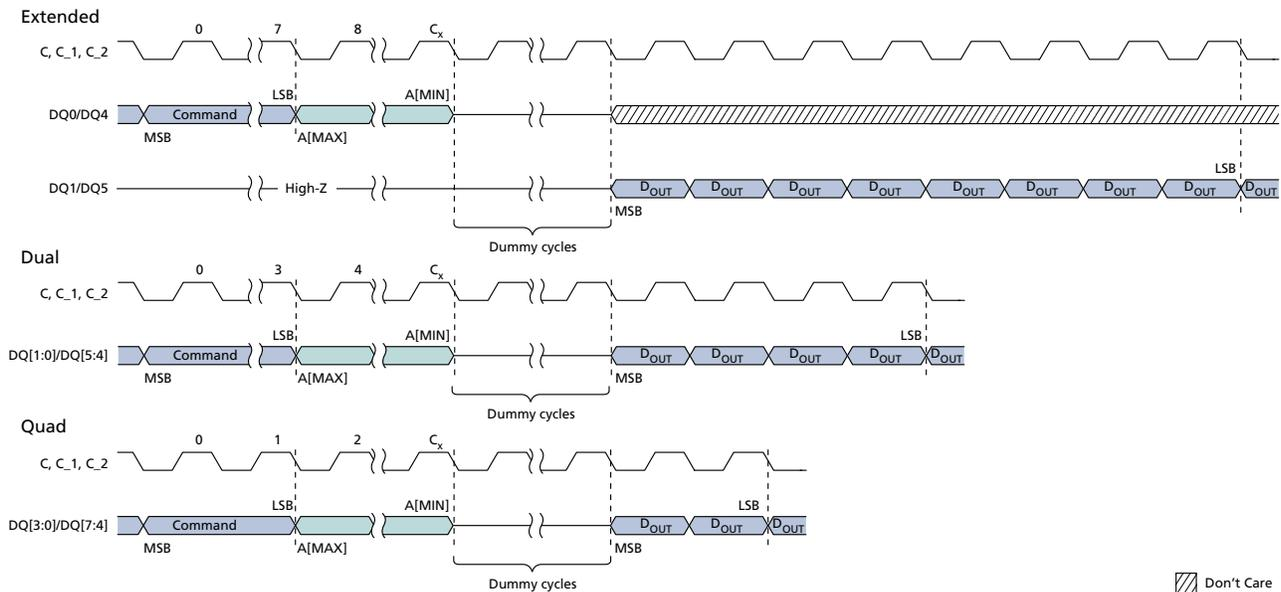
Note: 1. For extended SPI protocol,  $C_x = 7 + (A[\text{MAX}] + 1)$ ; For dual SPI protocol,  $C_x = 3 + (A[\text{MAX}] + 1)/2$ ; For quad SPI protocol,  $C_x = 1 + (A[\text{MAX}] + 1)/4$ .
