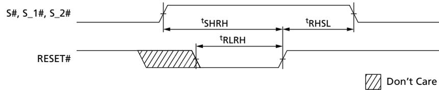
**Figure 48: Reset Enable and Reset Memory Timing**
