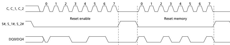
**Figure 49: Serial Input Timing**
