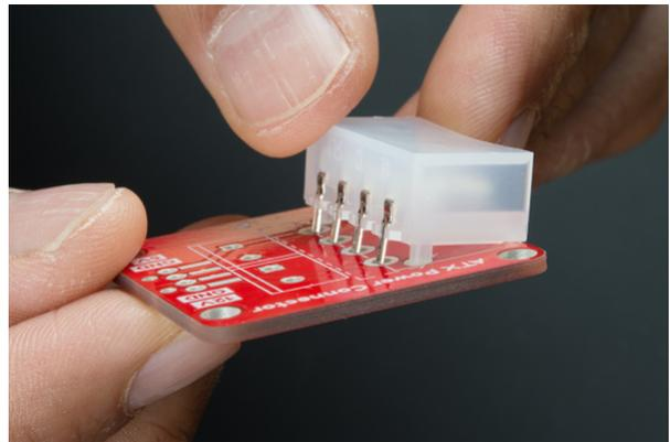
*Sliding Pins into Breakout*
