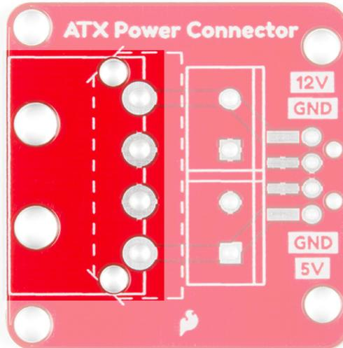
Depending on your application, you may want to add a vertical connector. Have no fear! The PTH pads were adjusted so that a 4-pin vertical connector can be added. Just follow the dashed silkscreen that outlines the perimeter of the connector.
