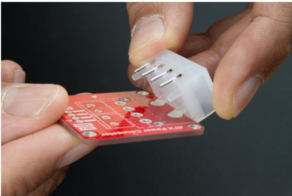
*Insert Support Leg into Breakout*
