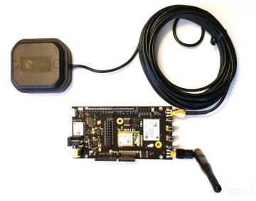
Figure 1: C099-F9P board and antennas
