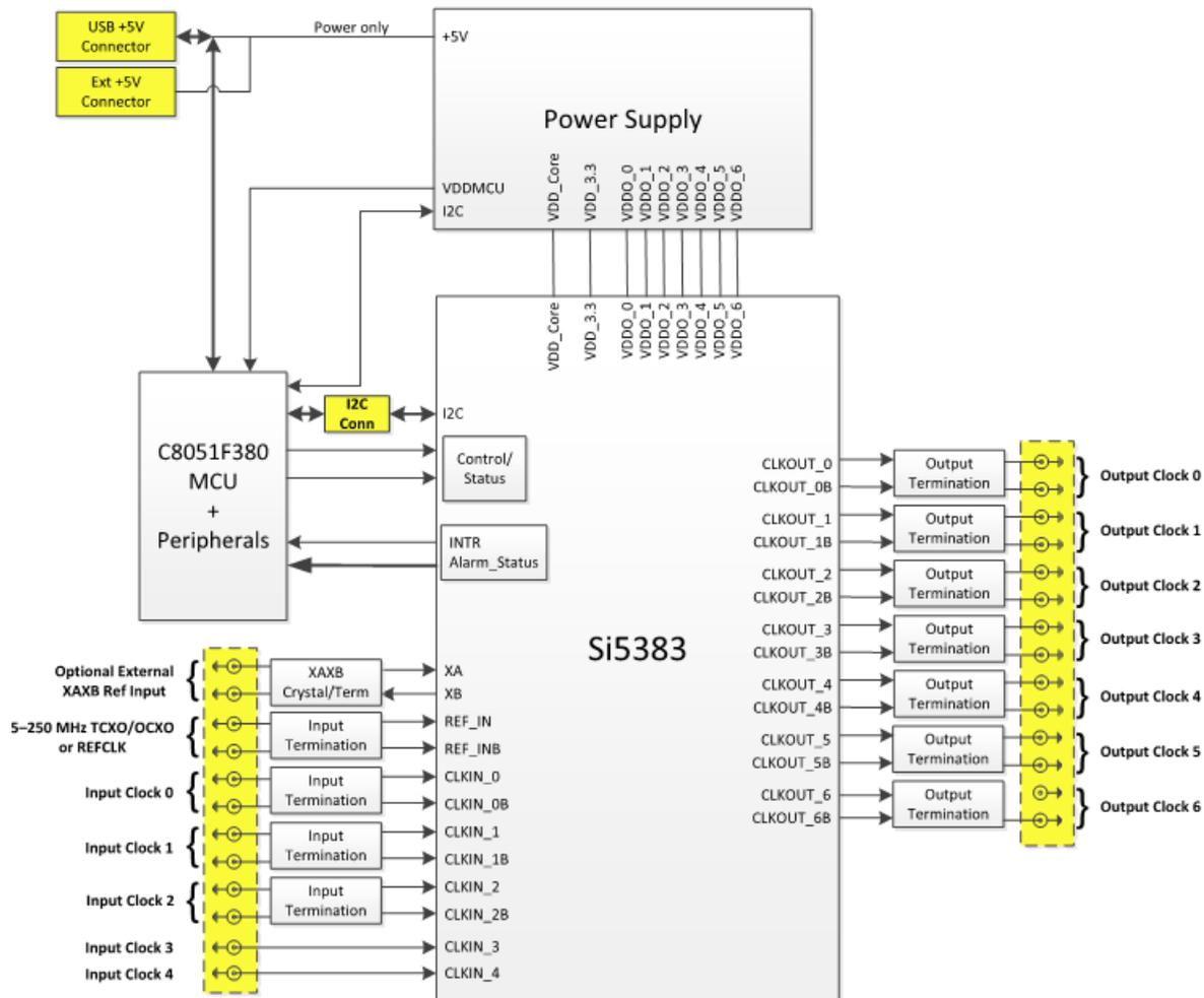
Figure 1.1. Si5383-EVB Functional Block Diagram
