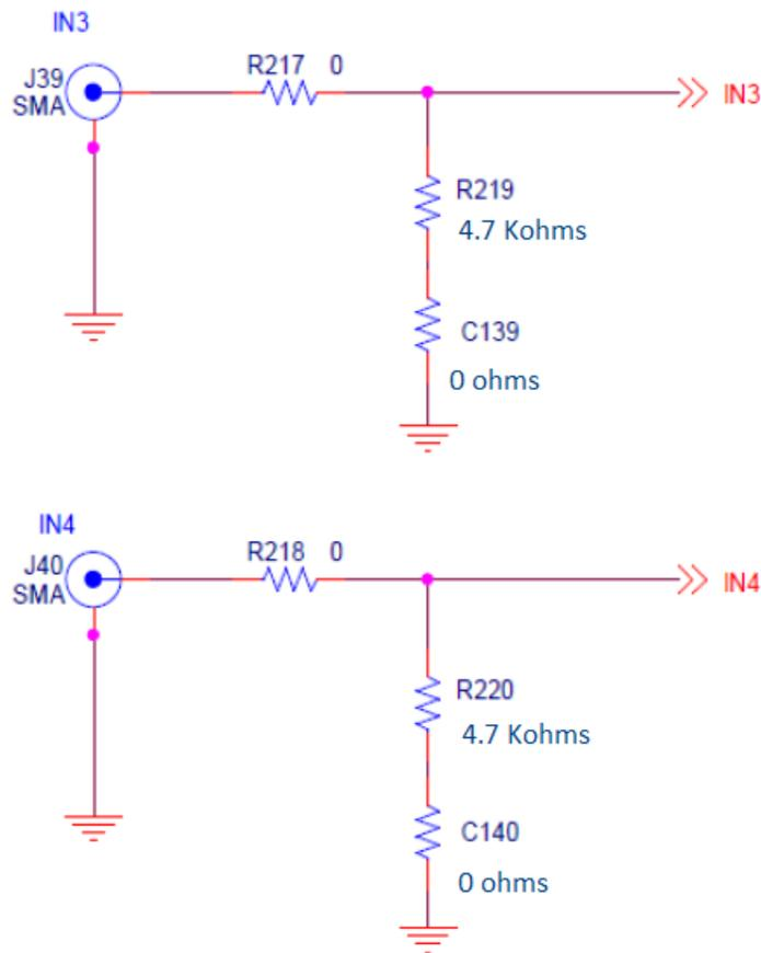
**Figure 5.3. IN3 and IN4, CMOS Input Terminations**
