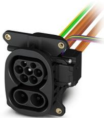
CHARX connect universal, Vehicle charging inlet, for charging with alternating current (AC) and with direct current (DC), CCS type 2, IEC 62196-2, IEC 62196-3, 250 A / 1000 V (DC), 32 A / 480 V (AC), Single wires, length: 2 m, locking actuator: 24 V, 4-pos., Front and rear mounting, M6, housing: black, A protective cap is supplied as standard for the DC and AC contacts.
