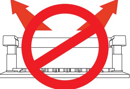
**Pull the actuator as horizontally as possible by a proper force**
