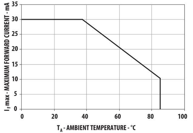
Figure 8. Maximum Forward Current vs Ambient Temperature
