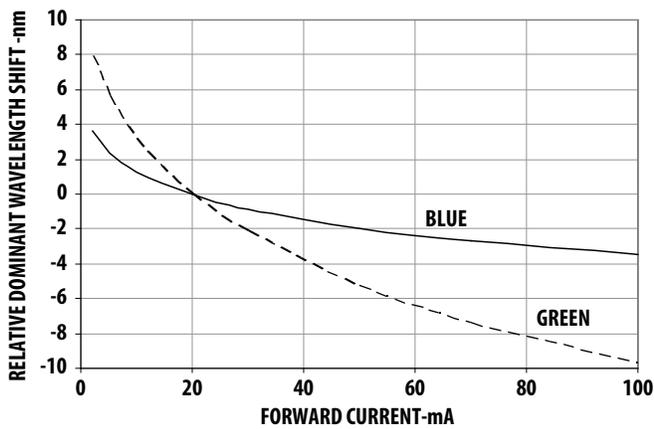
Figure 9. Relative dominant wavelength vs Forward Current
