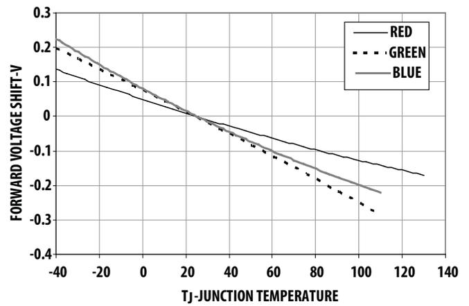
Figure 13. Relative Forward Voltage vs Junction Temperature
