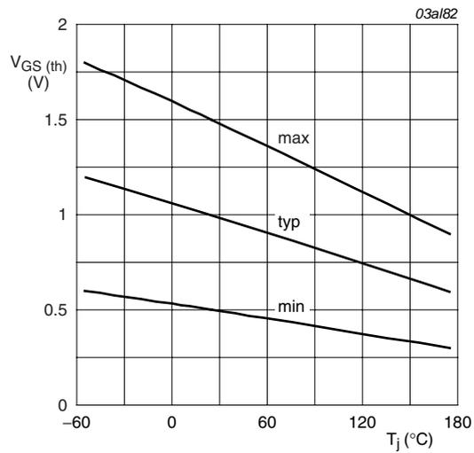
$I_D = 0.25 \text{ A}; V_{DS} = V_{GS}$
