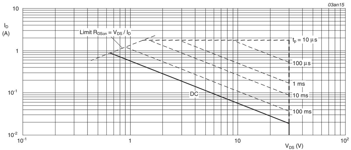
$T_{sp} = 25^\circ\text{C}$ ;  $I_{DM}$  is single pulse;  $V_{GS} = 4.5\text{V}$
