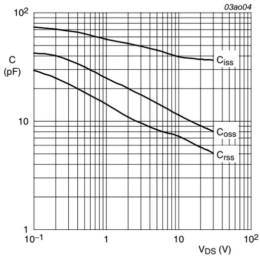
$V_{GS} = 0\text{ V}; f = 1\text{ MHz}$
