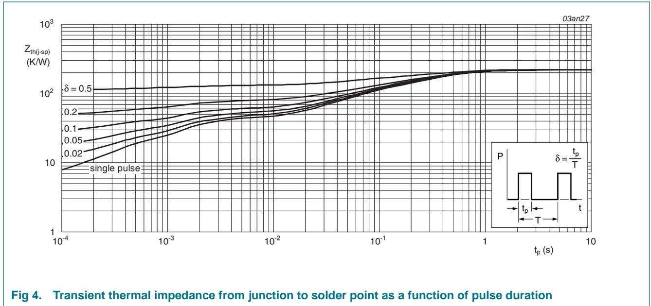
**Fig 4. Transient thermal impedance from junction to solder point as a function of pulse duration**
