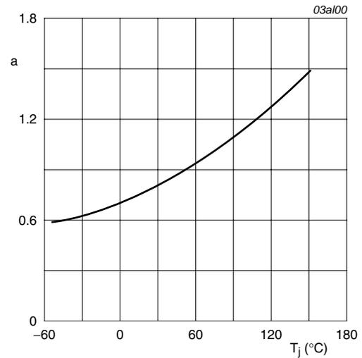
$$a = \frac{R_{DSon}}{R_{DSon(25^\circ\text{C})}}$$
