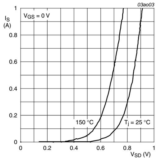
$T_j = 25\text{ }^\circ\text{C}$  and  $150\text{ }^\circ\text{C}; V_{GS} = 0\text{ V}$
