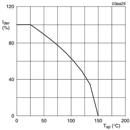
$$I_{der} = \frac{I_D}{I_{D(25^\circ\text{C})}} \times 100 \%$$
