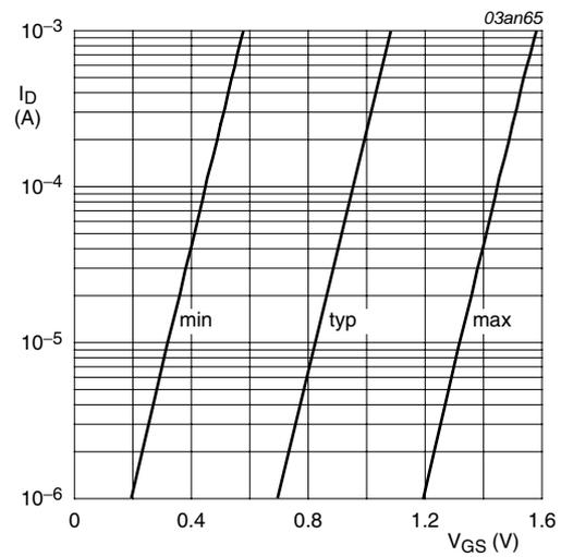
$T_j = 25^\circ\text{C}; V_{DS} = 5 \text{ V}$
