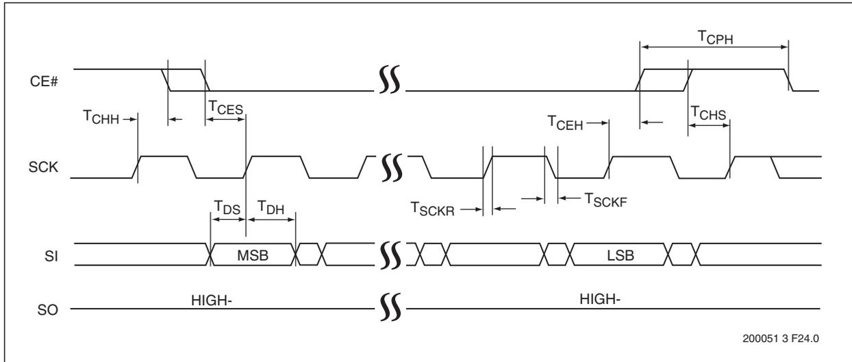
FIGURE 6-4: SERIAL INPUT TIMING DIAGRAM
