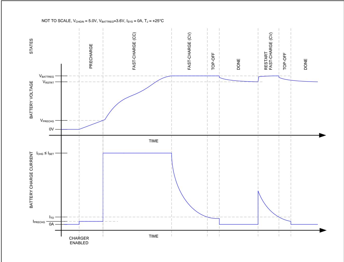
Figure 7. LiFePO<sub>4</sub> Battery Charge Profile
