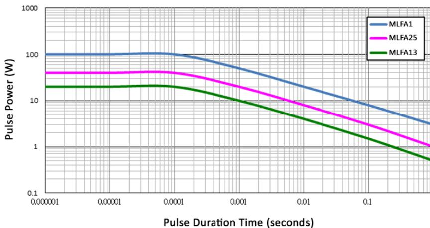
**MLFA Series Continuous Pulse ( $R \geq 10 \text{ ohm}$ )**
