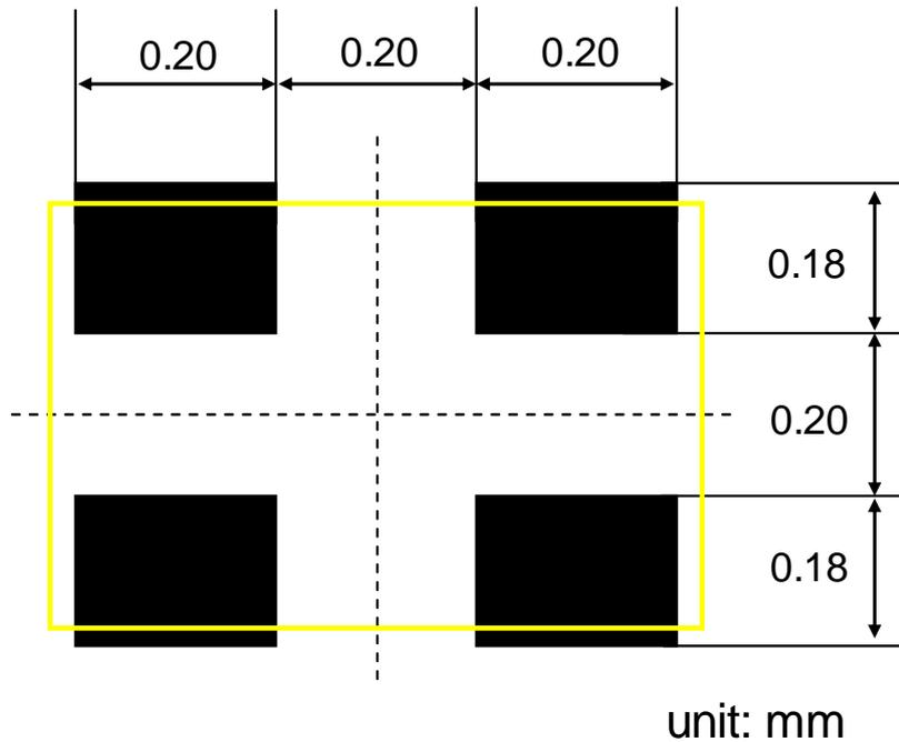
Line width be designed to match 50 ohm characteristic impedance depending on PCB Material and thickness.
