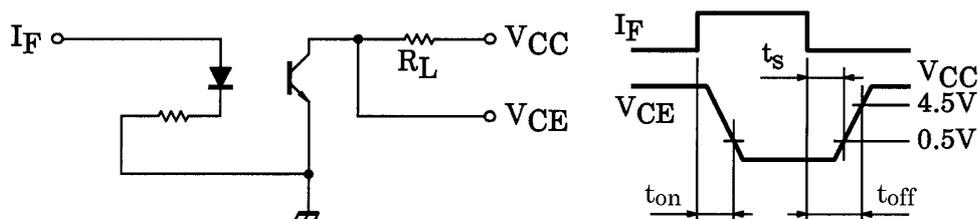
**Fig. 11.1 Switching Time Test Circuit and Waveform**
