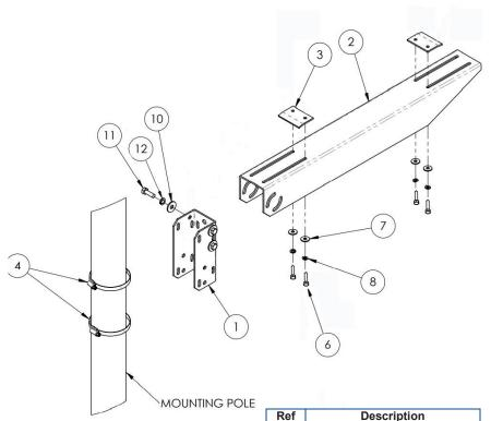
**STEP 3:** Attach the two solar panel clamps to the arm using four 6mm bolts, washers and lock-washers. The clamping edges should be pointing away from each other. Don't tighten at this point, leave them loose.
