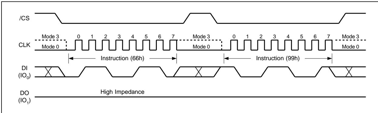
Figure 5b. Enable Reset and Reset Instruction Sequence
