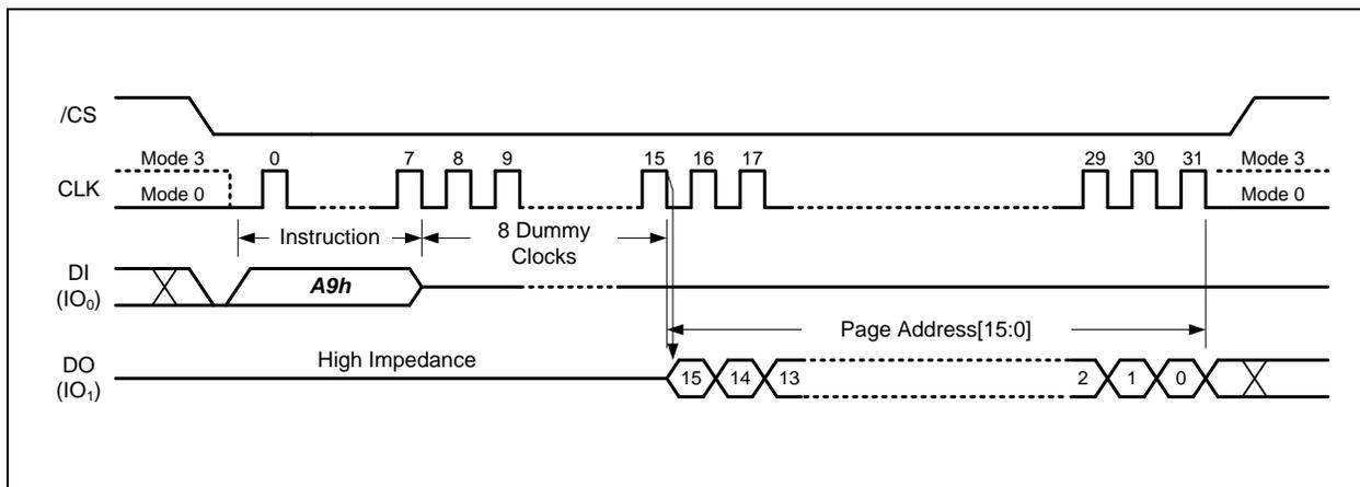
Figure 13. Last ECC Failure Page Address Instruction
