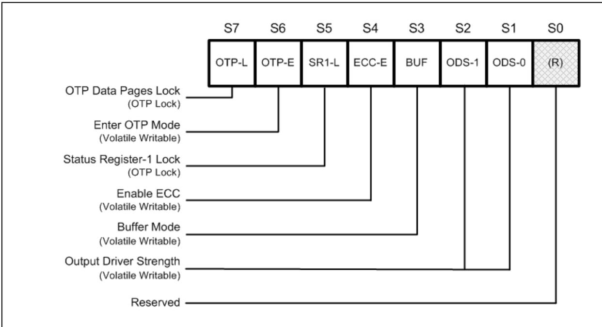
Figure 3b. Configuration Register / Status Register-2 (Address Bxh)
