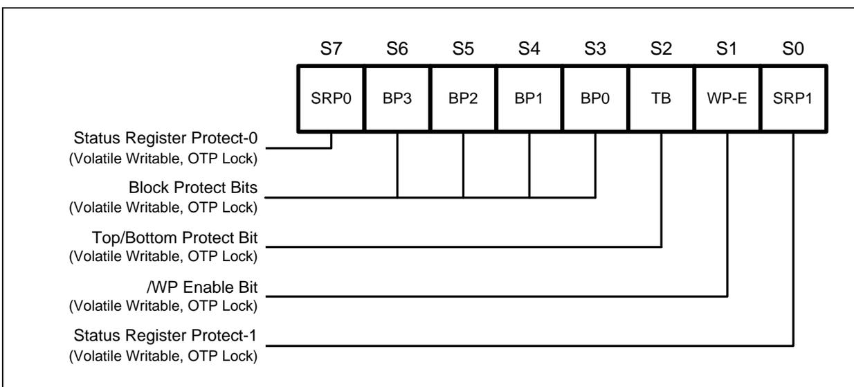
Figure 3a. Protection Register / Status Register-1 (Address Axh)
