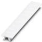
Zack marker strip, Strip, white, labeled, can be labeled with: Plotter, Printed horizontally: Consecutive numbers 1 - 10, 11 - 20, etc. up to 491 - 500, Mounting type: Snap into tall marker groove, for terminal block width: 6.2 mm, Lettering field: 6.15 x 10.5 mm
