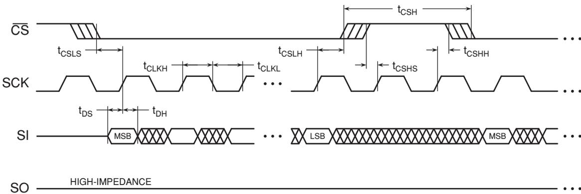
Figure 15-2. Serial Output Timing
