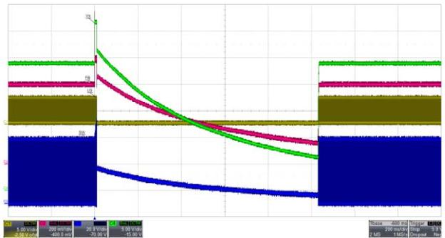
Figure 33. OVP2 Release at  $V_{FB} \leq 100\% V_{REF}$
