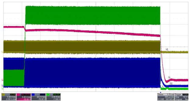
Figure 27. Over-current Protection with 280 kHz Switching Frequency
