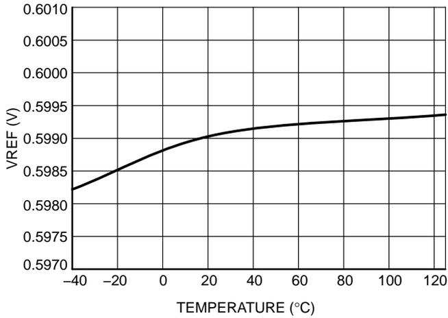
Figure 10.  $V_{REF}$  vs T at  $V_{HVBIAS} = 48\text{ V}$
