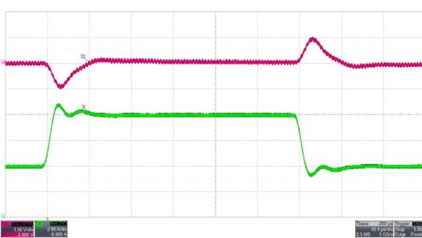
**Figure 36. Load Step between 50% and 100% Load**
