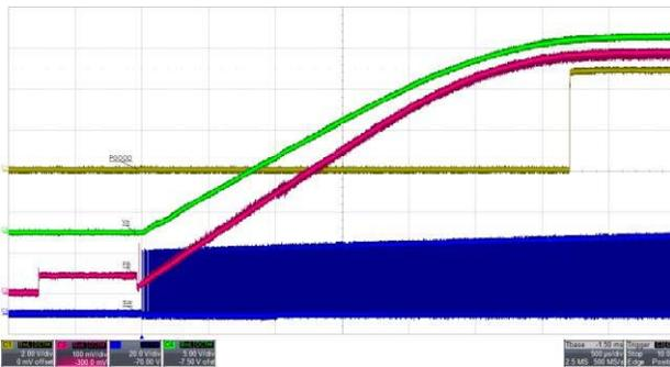
Figure 28. Power Good at Startup with No Load
