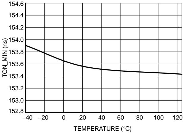
Figure 18.  $T_{ON\_MIN}$  vs. T at  $V_{HVBIAS} = 48\text{ V}$
