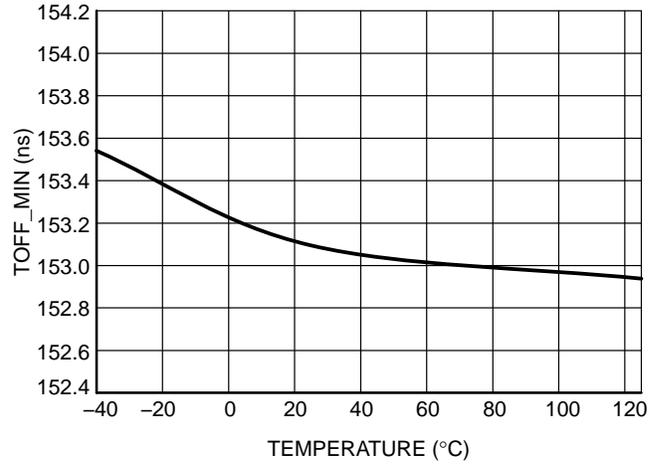
Figure 19.  $T_{OFF\_MIN}$  vs. T at  $V_{HVBIAS} = 48\text{ V}$
