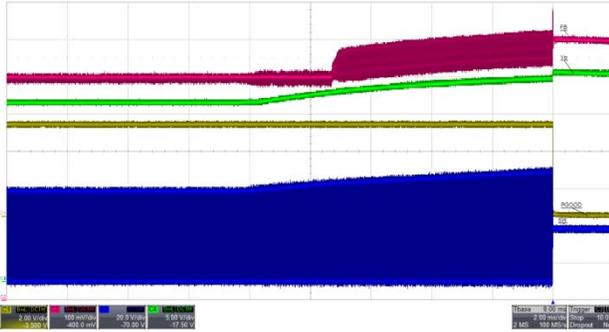
Figure 30. OVP1 at  $V_{FB} \geq 115\% V_{REF}$
