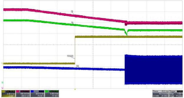
Figure 31. OVP1 Release at  $V_{FB} \leq 110\% V_{REF}$
