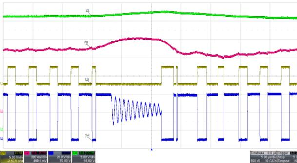
Figure 32. OVP2 at  $V_{FB} \geq 130\% V_{REF}$
