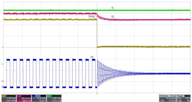
Figure 29. Power Good at Startup with No Load
