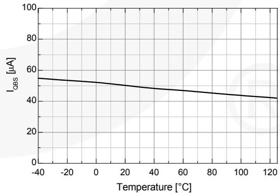
Figure 15. Quiescent V<sub>BS</sub> Supply Current vs. Temperature
