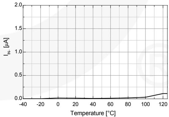
Figure 27. Logic Input LOW Bias Current vs. Temperature
