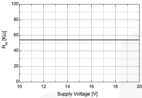
Figure 28. Input Pull-Down Resistance vs. Supply Voltage
