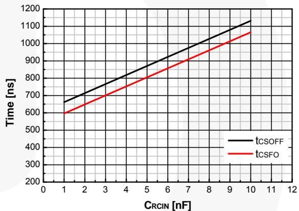
Figure 43. Timing of  $t_{CSOFF}$  and  $t_{CSFO}$  vs.  $C_{RCIN}$
