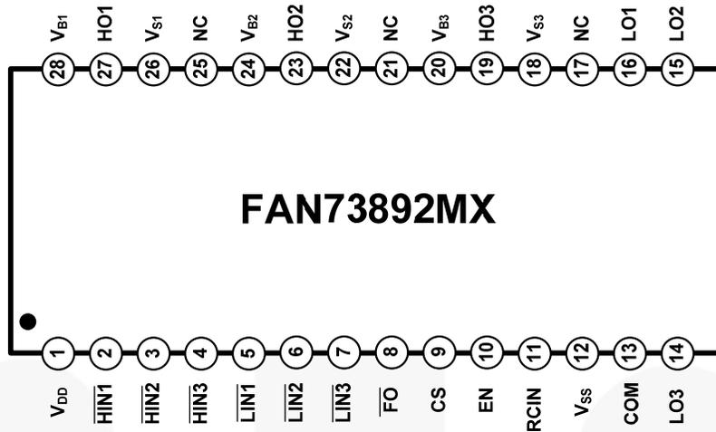
Figure 3. Pin Assignments
