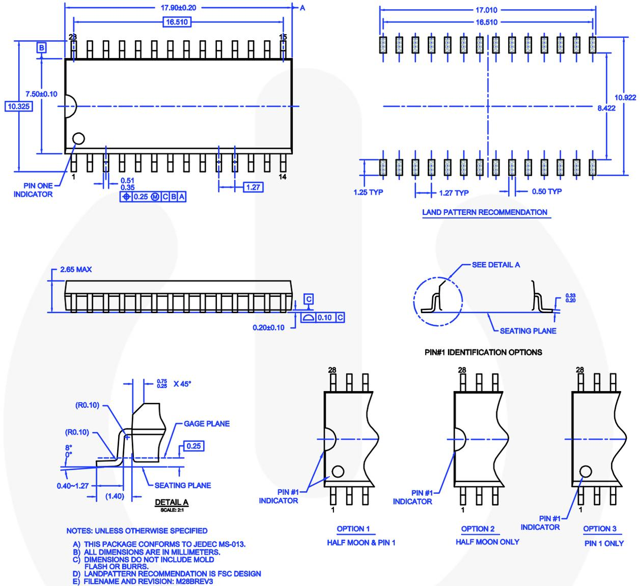
**Figure 47. 28-Lead, Small Outline Integrated Circuit, (28 Wide-Body SOIC)**
