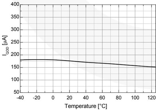
Figure 14. Quiescent V<sub>DD</sub> Supply Current vs. Temperature
