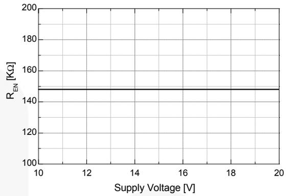
Figure 29. Enable Pin Pull-Down Resistance vs. Supply Voltage
