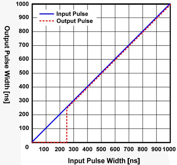
Figure 46. Input Filter Characteristic of Narrow ON
