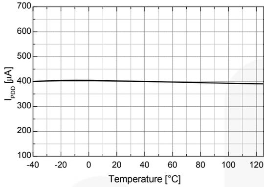
Figure 16. Operating  $V_{DD}$  Supply Current vs. Temperature
