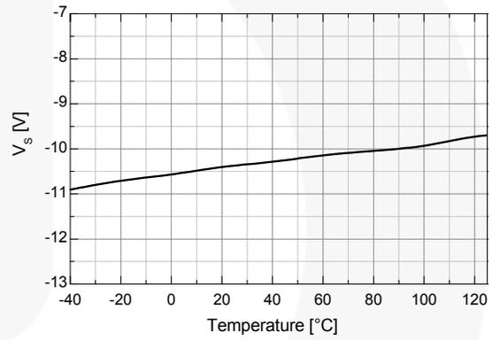
Figure 13. Allowable Negative V<sub>S</sub> Voltage vs. Temperature
