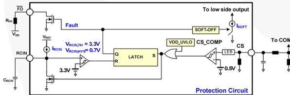
Figure 41. Over-Current Protection
