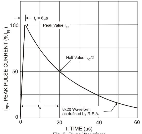
Fig. 6 Pulse Waveform
