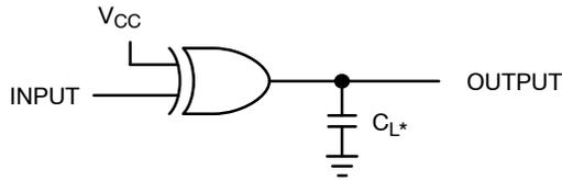
\*Includes all probe and jig capacitance.
