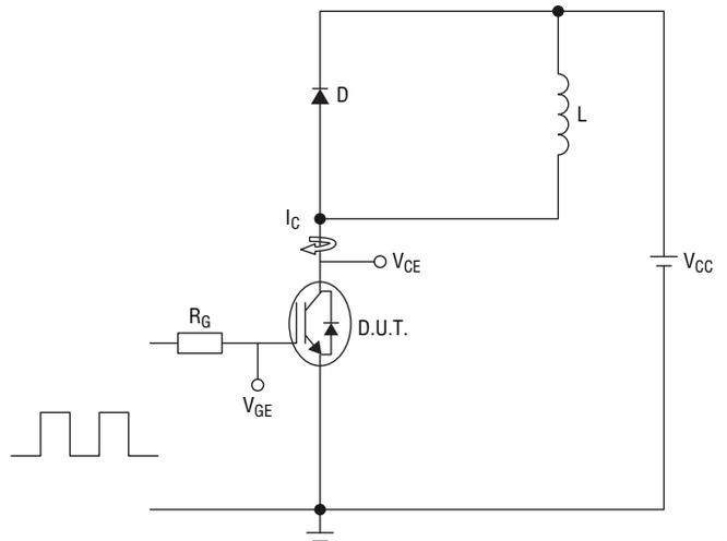
$L = 1.87 \text{ mH}$ ,  $V_{CE} = 400 \text{ V}$ ,  $V_{GE} = 15 \text{ V}$ ,  $I_C = 30 \text{ A}$ ,  $R_G = 10 \Omega$
