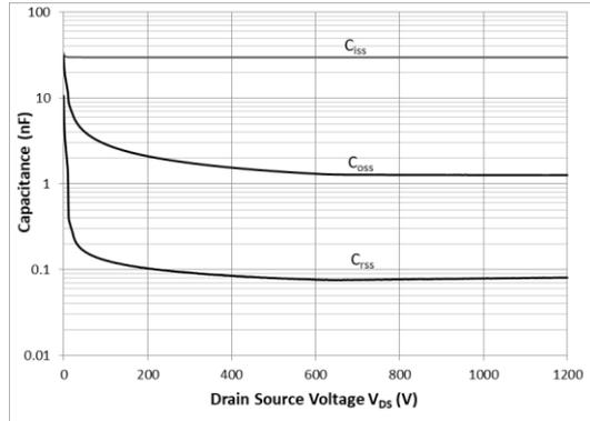
**Figure 8:** Typical capacitances vs  $V_{DS}$
