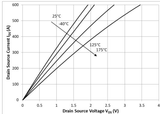
**Figure 1:** Drain current vs  $V_{DS}$
