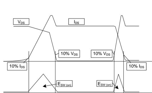
**Figure 14:** Switching energy computation
