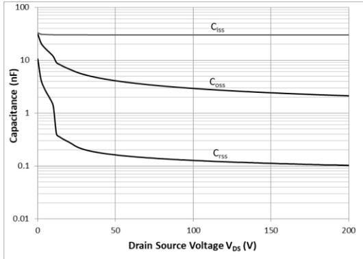
**Figure 7:** Typical capacitances vs  $V_{DS}$
