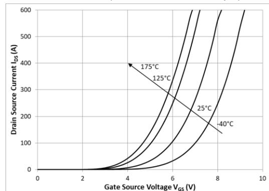
**Figure 4:** Drain current vs  $V_{GS}$  voltage
