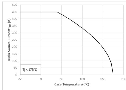
**Figure 18:** Continuous Drain Current Derating vs Case temperature
