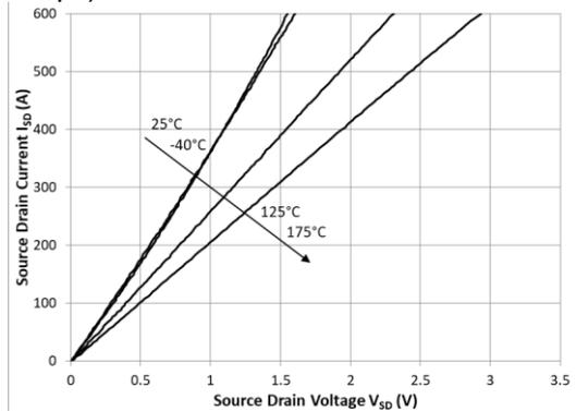
**Figure 5 :** 3rd quadrant characteristics
