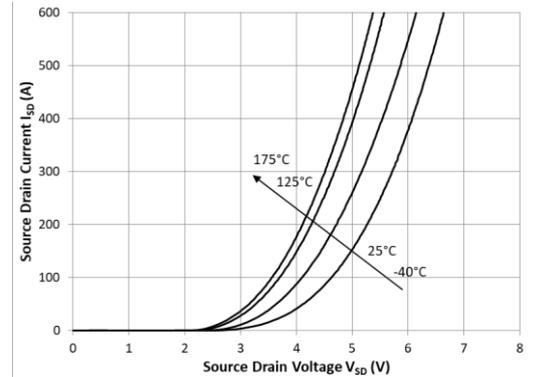
**Figure 6:** 3rd quadrant characteristics
