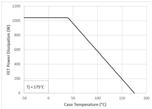
**Figure 19 :** Maximum Power Dissipation Derating vs Case temperature
