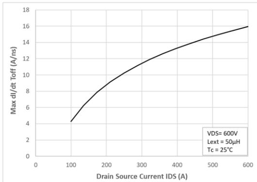
**Figure 13:** Max Turn-off  $di/dt$  vs Drain current
