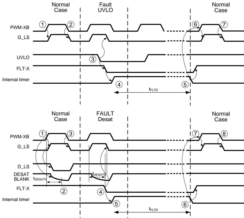
**Figure 26: Timing diagram CXT-PLA3SA12450A low-side gate driver behaviour**
