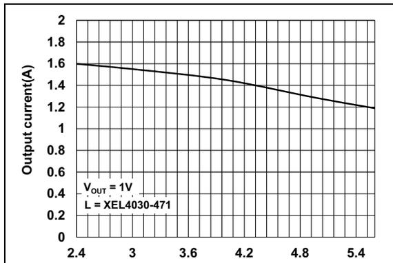
**FIGURE 2-8:** DCM/FPWM  $I_{OUT}$  Threshold vs.  $V_{IN}$ .
