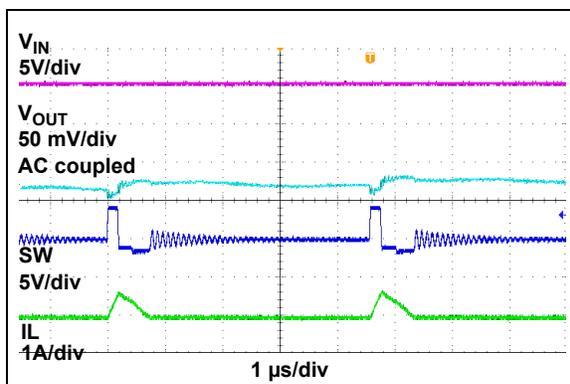
**FIGURE 2-21:** Switching Waveforms,  $I_{OUT} = 50 mA$ .
