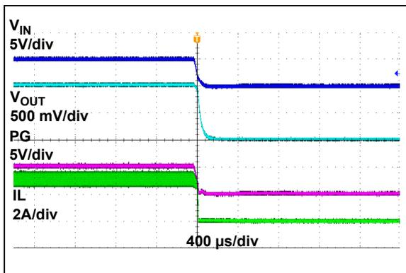
FIGURE 2-14:  $V_{IN}$  Turn-Off ( $EN = PV_{IN}$ ),  $R_{LOAD} = 0.3\Omega$ .
