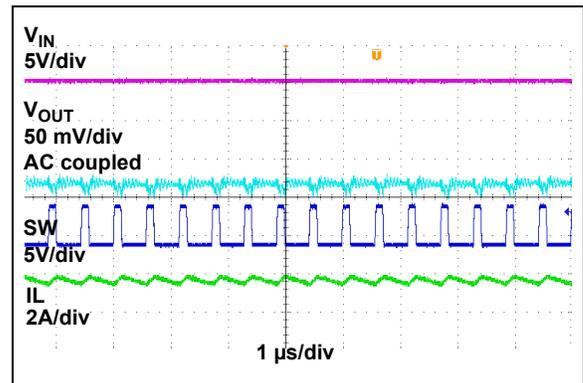
**FIGURE 2-22:** Switching Waveforms,  $I_{OUT} = 6A$ .
