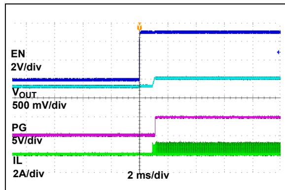
FIGURE 2-17:  $EN$  Turn-On into Pre-Biased Output ( $V_{pre-bias} = 0.8V$ ).
