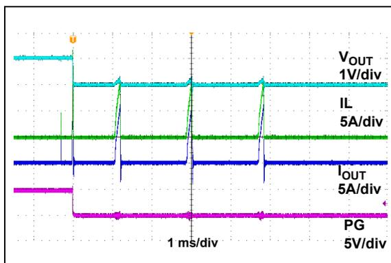
**FIGURE 2-20:** Hiccup Mode Short-Circuit Current Limit Response.
