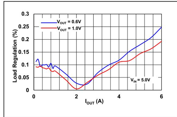
**FIGURE 2-10:** Load Regulation:  $V_{OUT}$  Voltage Variation vs.  $I_{OUT}$ .
