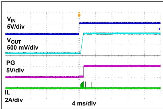
FIGURE 2-13:  $V_{IN}$  Turn-On ( $EN = PV_{IN}$ ).
