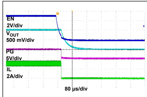
FIGURE 2-16:  $EN$  Turn-Off,  $R_{LOAD} = 0.3\Omega$ .
