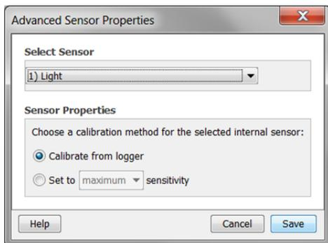
**Note:** The sensor is sensitive to lights that emit high amounts of infrared radiation like incandescent and halogen bulbs. It is best to use auto-calibration when possible when monitoring on/off conditions for lights with high infrared radiation.
