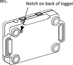
2. Insert the black base of the attachment into the notch so that the base clips onto the corner of the logger as shown below.
