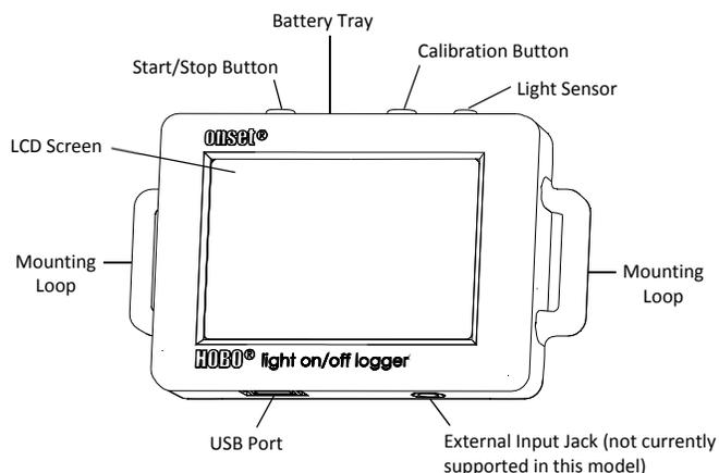
**Start/Stop Button:** Press this button for 3 seconds to start or stop logging data. This requires configuring the logger in HOBOWare with a push button start or stop (see *Setting up the Logger*). You can also press this button for 1 second to record an internal event (see *Recording Internal Logger Events*) or to turn the LCD screen on if the option to turn off the LCD has been enabled (see *Setting up the Logger*).
