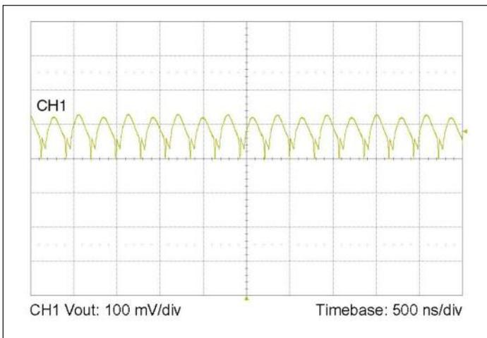
Figure 5 — Output voltage ripple at full load and 48 V<sub>F</sub> with no POL bypass capacitance.
