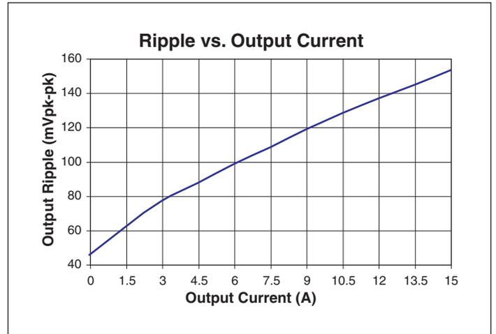
Figure 2 — Output voltage ripple vs. output current at 48 V<sub>F</sub> with no POL bypass capacitance.
