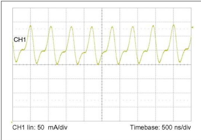
Figure 1 — Input reflected ripple current at full load and 48 V<sub>F</sub>.
