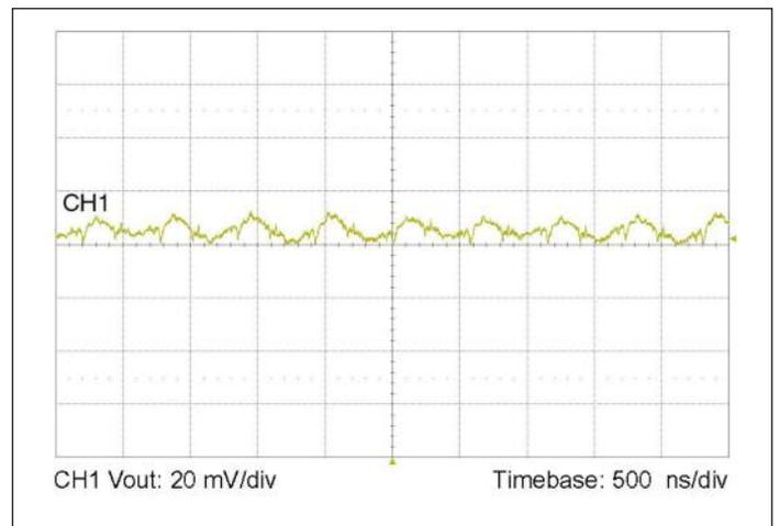
Figure 6 — Output voltage ripple at full load and 48 V<sub>F</sub> with 10 μF ceramic POL bypass capacitance and 20 nH distribution inductance.
