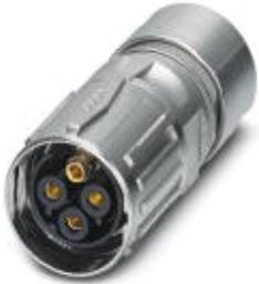
Cable connector, straight, SPEEDCON locking, M17, Number of positions: 5+PE, Type of contact: Socket, Crimp connection, shielded: yes, Cable diameter: 3.5 mm...5.5 mm
