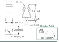
\*Fuse clips without end stops are not UL recognized
