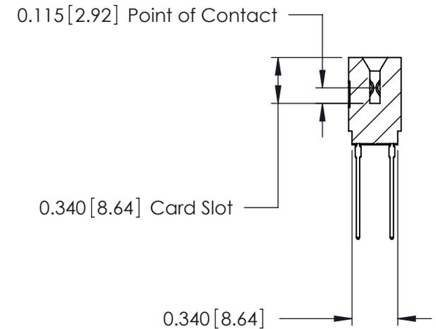
746 Series Ultra-Mate Card Edge Connector - Press Fit
