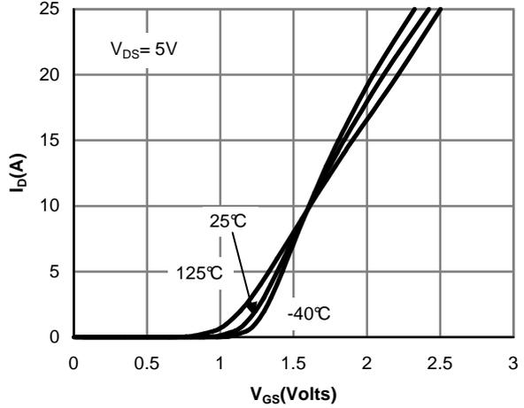
Figure 2: Transfer Characteristics
