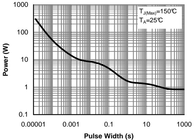
Figure 10: Single Pulse Power Rating Junction-to-Ambient (Note E)
