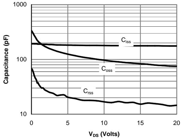
Figure 8: Capacitance Characteristics
