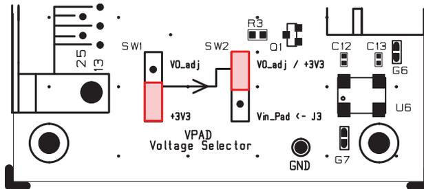
SW2 is in VO\_adj/+3V3 position. SW1 is in +3V3 position.
