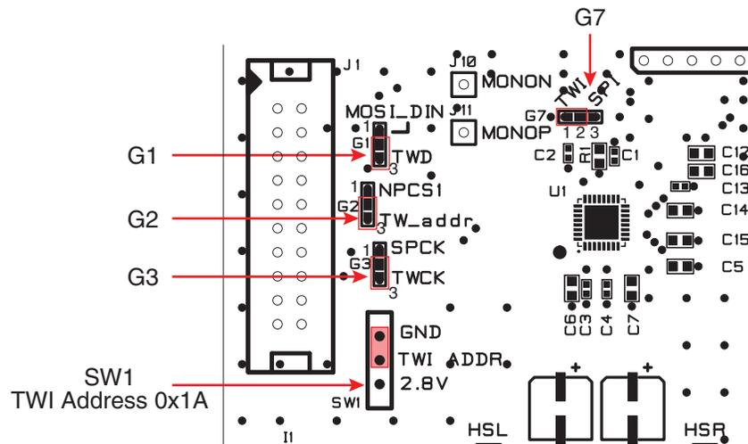
**Figure 2-13.** TWI Address Switch (SW1) - Case Address = 1
