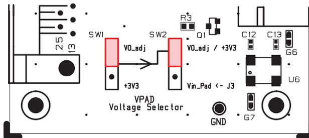
SW2 is in VO\_adj/+3V3 position. SW1 is in VO\_adj position.
