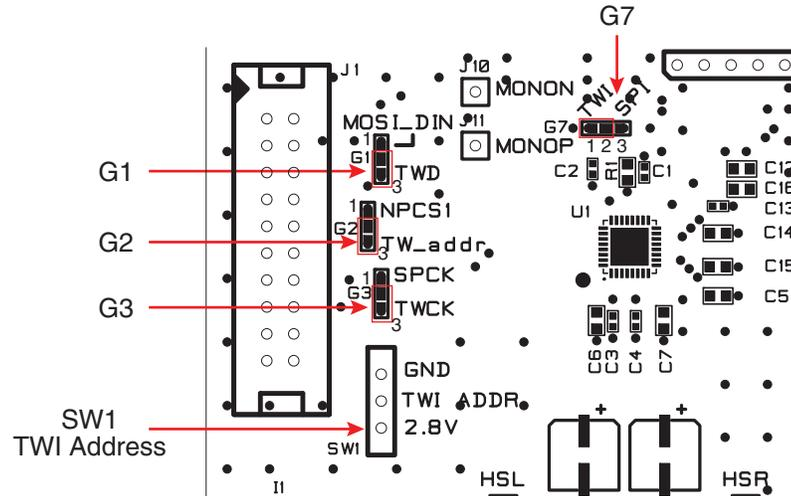
**Figure 2-12.** TWI Address Switch (SW1) - Case Address = 0
