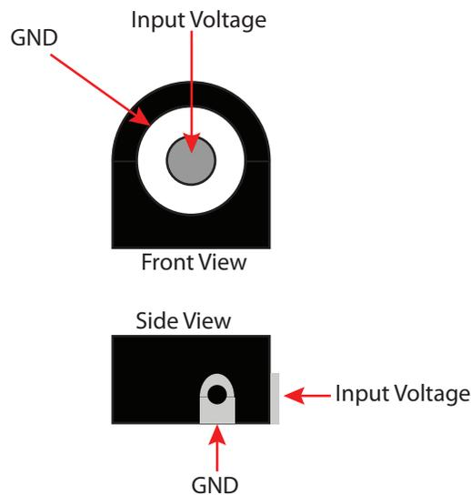
If chosen as an alternative, connect the power supply (+) to Vin test-point (TP1) and (-) to GND test-point (TP2 or TP3).
