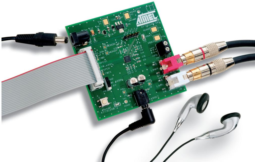
Figure 1-3. AT73C240-EK1 Components Side
