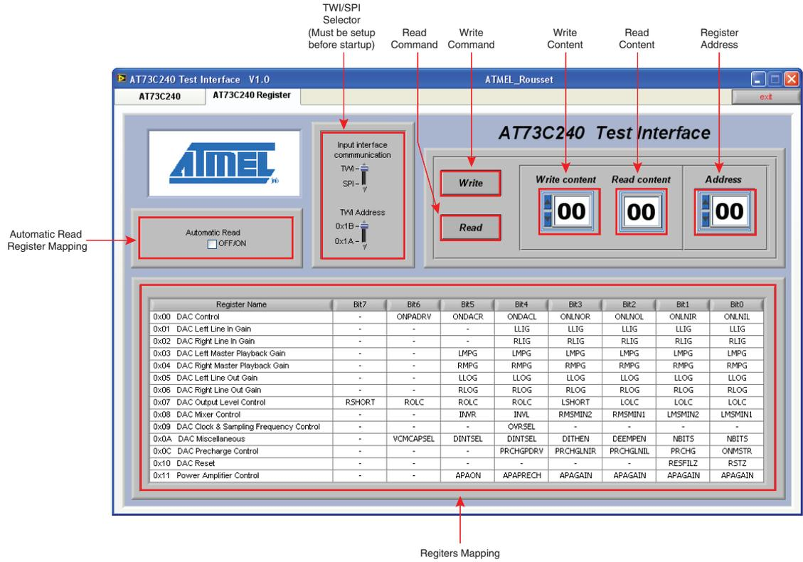
**Note:** Resetting all the registers done by pressing once on the AT73C240 Reset push-button I2. In the next read action the registers will be at their default values.
