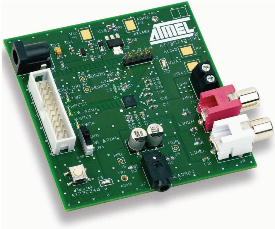
The AT73C240 is located in the center of the AT73C240-EK1 on the Components Side.
