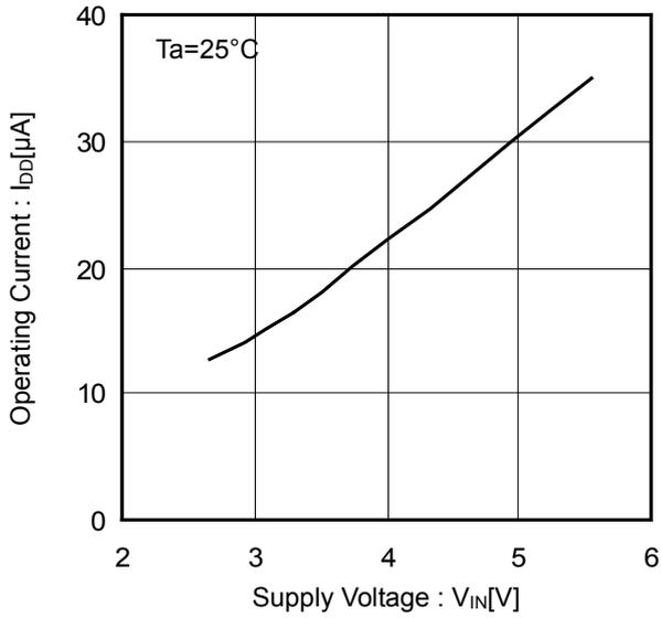
Figure 1. Operating Current vs Supply Voltage (EN Enable)
