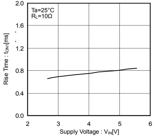
Figure 10. Output Rise Time vs Supply Voltage
