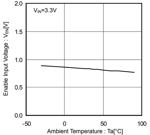
Figure 6. EN Input Voltage vs Ambient Temperature
