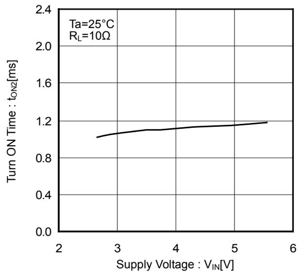
Figure 12. Output Turn ON Time vs Supply Voltage
