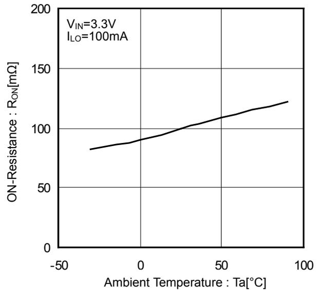
Figure 8. ON-Resistance vs Ambient Temperature
