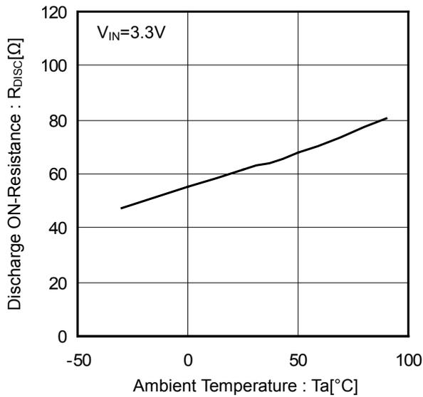
Figure 19. Discharge ON-Resistance vs Ambient Temperature
