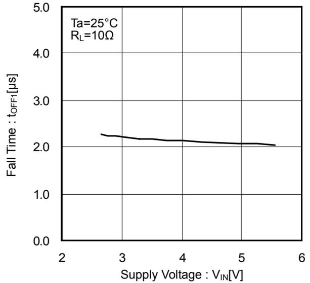
Figure 14. Output Fall Time vs Supply Voltage
