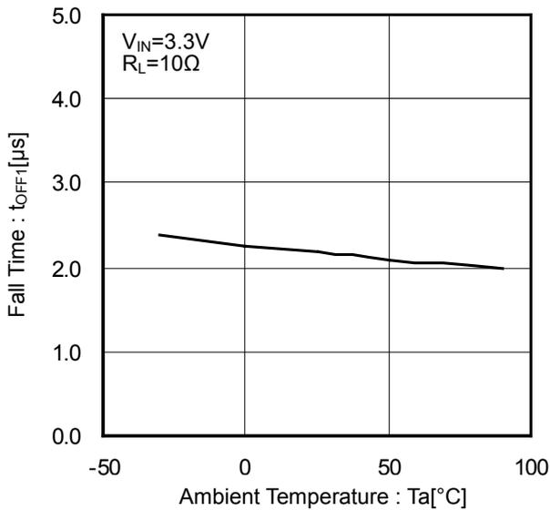
Figure 15. Output Fall Time vs Ambient Temperature
