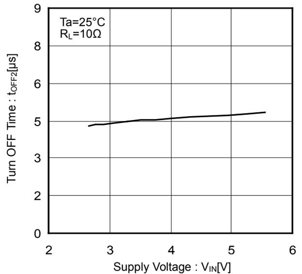
Figure 16. Output Turn OFF Time vs Supply Voltage
