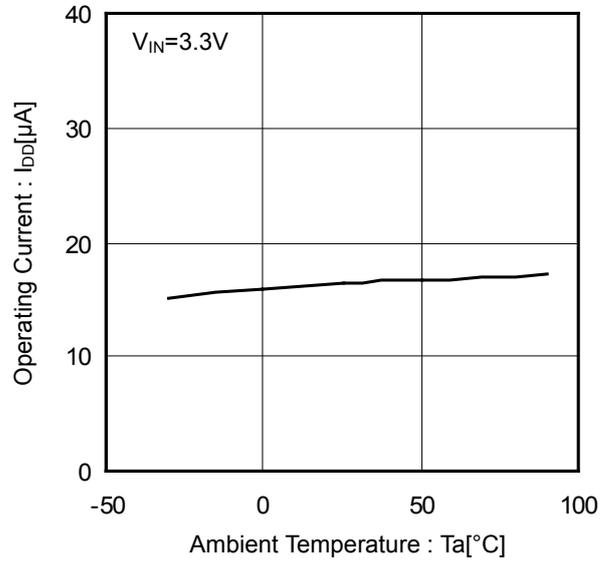
Figure 2. Operating Current vs Ambient Temperature (EN Enable)
