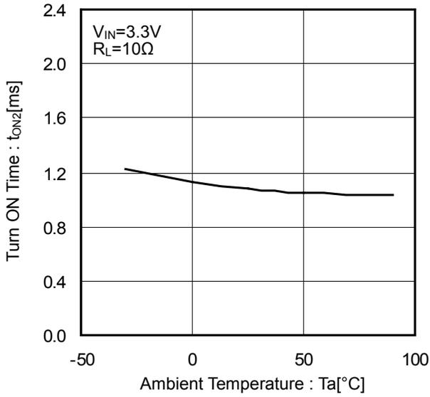
Figure 13. Output Turn ON Time vs Ambient Temperature
