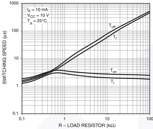
Figure 9. Switching Speed vs. Load Resistor
