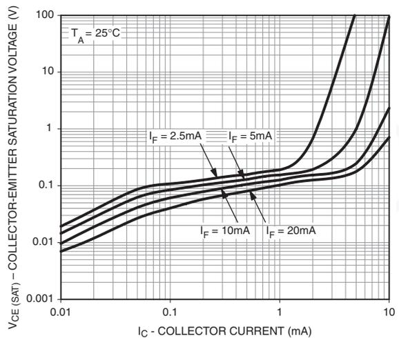
Figure 8. Collector-Emitter Saturation Voltage vs. Collector Current
