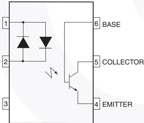
Figure 1. Schematic
