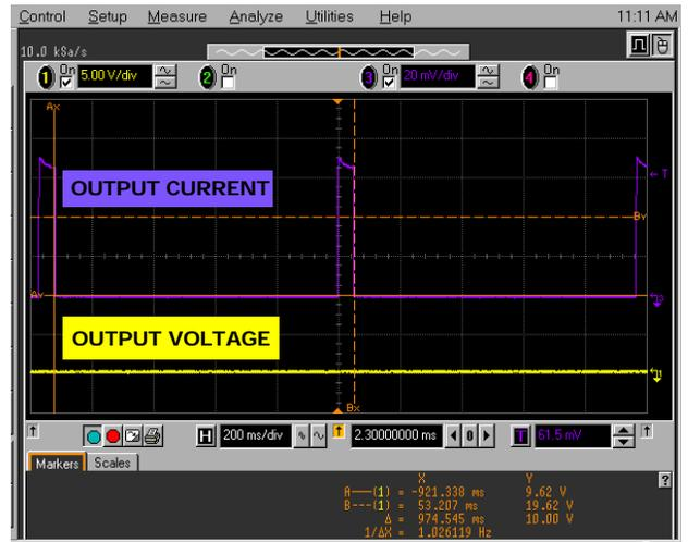
FIGURE 15. VLNb SHORTED TO GND, 200mA<sup>2</sup>
