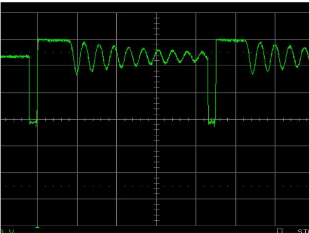
FIGURE 6. BOOST SWITCH NODE AT 0A (DISCONTINUOUS)
