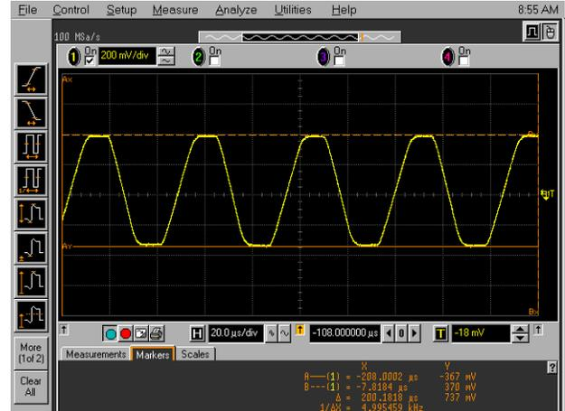
FIGURE 11. 22kHz TONE ON 13.3V<sub>OUT</sub> WITH 50mA LOAD
