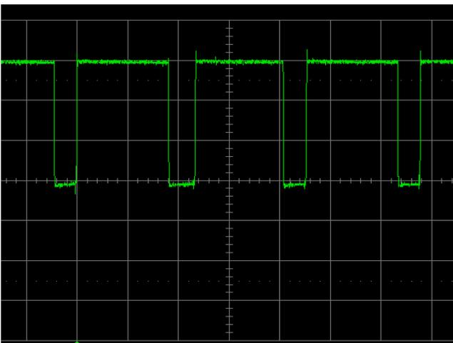
FIGURE 8. BOOST SWITCH NODE AT 300mA (CONTINUOUS MODE)
