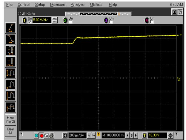
FIGURE 9. V\_LNB TRANSITIONS FROM 13.3V TO 18.3V
