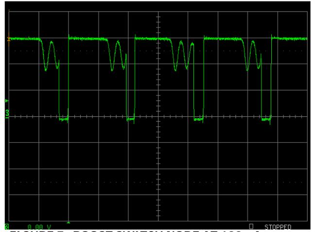
FIGURE 7. BOOST SWITCH NODE AT 100mA (PARTIAL CONTINUOUS)
