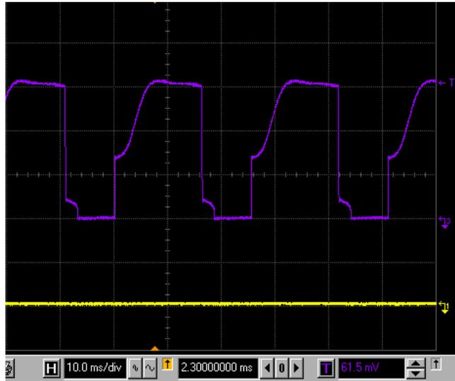
FIGURE 18. THE ISL9491 IN THERMAL EQUILIBRIUM WITH  $R_{ILIM} = 0$
