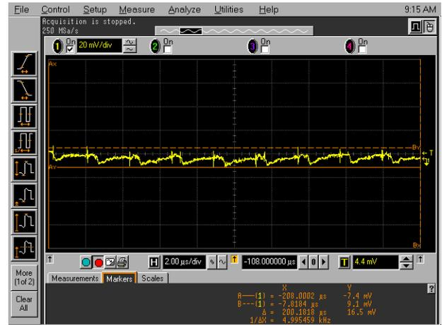
FIGURE 13. AC NOISE ON 13.3V<sub>OUT</sub> AT 500mA OF LOAD
