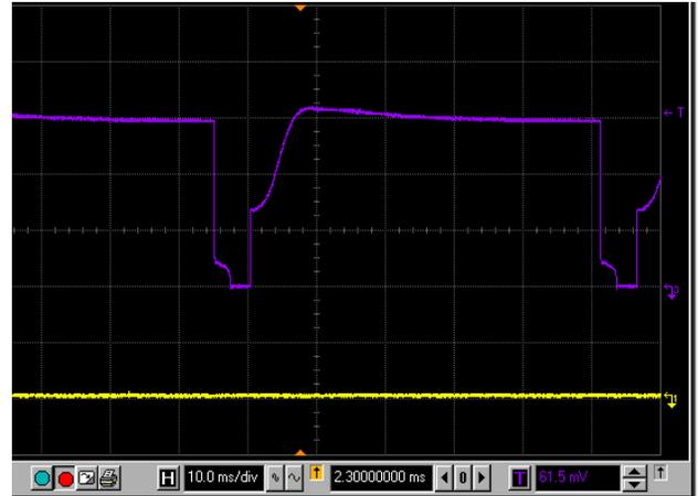
FIGURE 17. THE ISL9491 ENTERING THERMAL SHUTDOWN WITH  $R_{ILIM} = 0$
