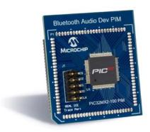
The PIC32MX254F256 Bluetooth Audio PIM is designed to demonstrate the capabilities of the PIC32MX XLP family of devices using the PIC32 Bluetooth Audio Development Kit. It enables Bluetooth and Digital Audio development with PIC32 Bluetooth Audio Development Kit.
