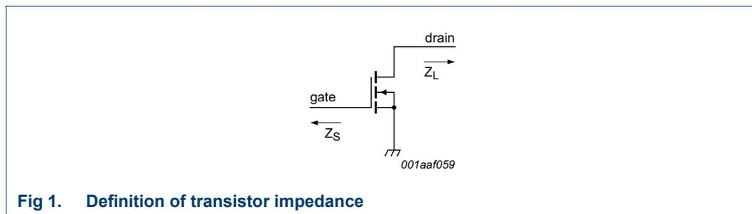
**Fig 1. Definition of transistor impedance**
