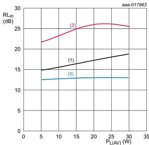
$V_{DS} = 28\text{ V}$ ;  $I_{Dq} = 300\text{ mA}$  (main device);  $V_{GS(amp)peak} = 0.7\text{ V}$ .
