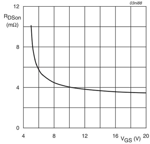
$T_j = 25^\circ\text{C}; I_D = 50\text{A}$
