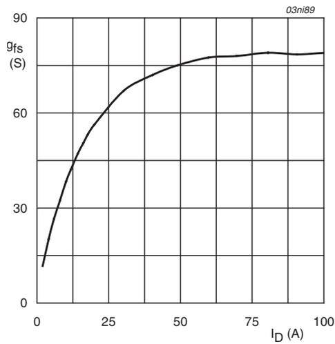
$T_j = 25^\circ\text{C}; V_{DS} = 25\text{V}$
