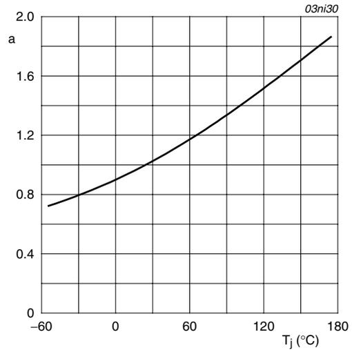
$$a = \frac{R_{DSon}}{R_{DSon(25^\circ\text{C})}}$$
