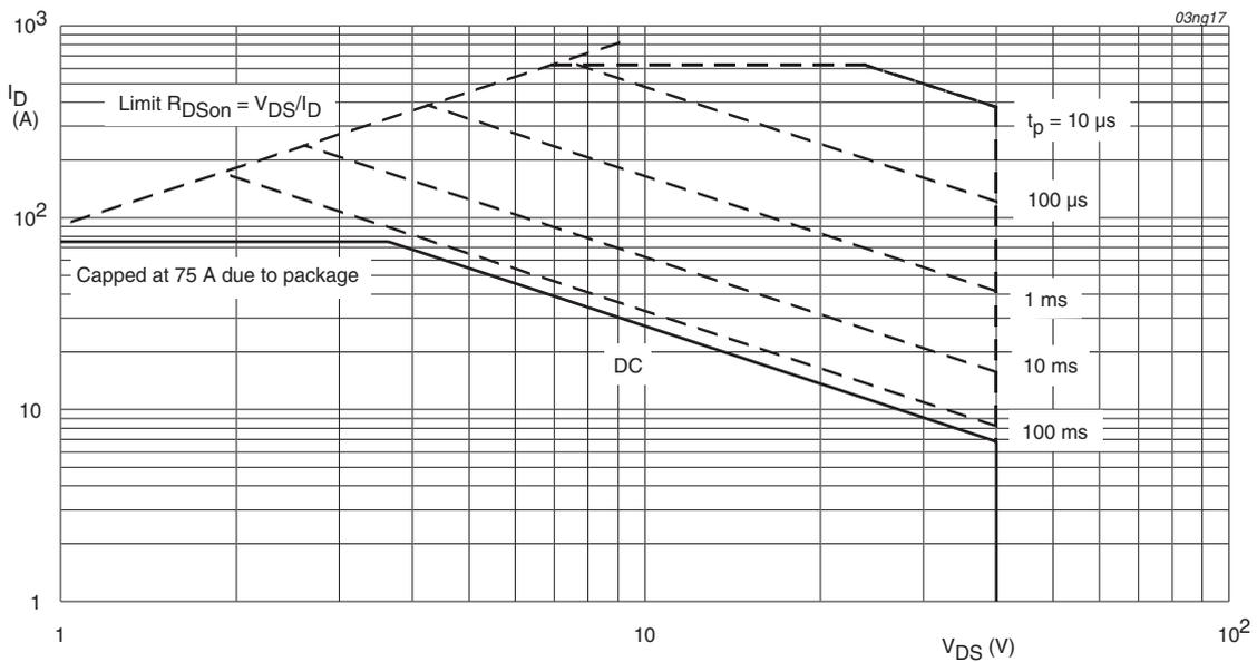
$T_{mb} = 25^{\circ}C; I_{DM}$  is single pulse
