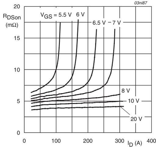
$T_j = 25^\circ\text{C}; t_p = 300\mu\text{s}$
