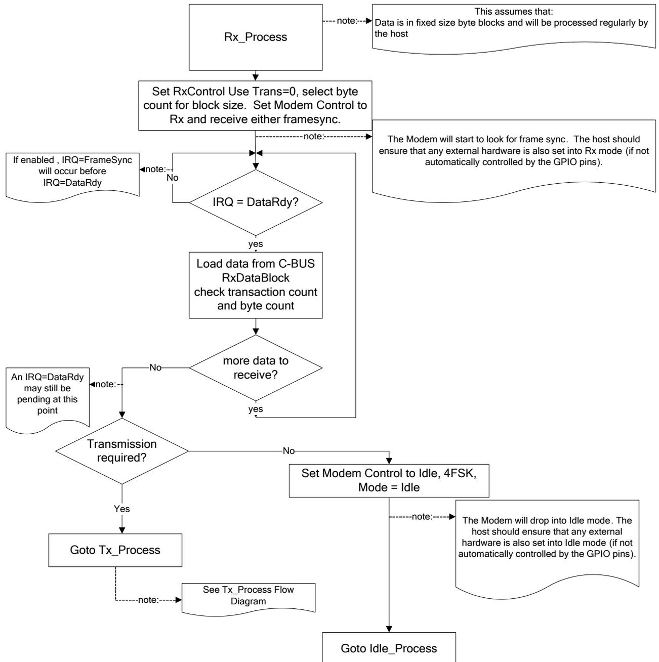
Figure 8 Host Rx Data Flow (Use Trans=0)
