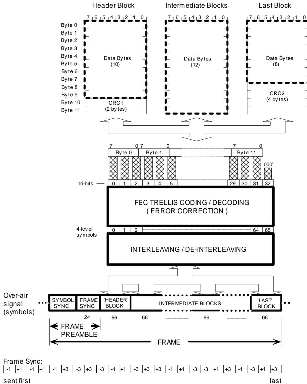
Figure 15 Formatted Data Over Air Signal Format
