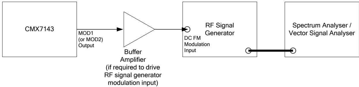
**Figure 18 Tx Spectrum and Modulation Measurement Configuration**
