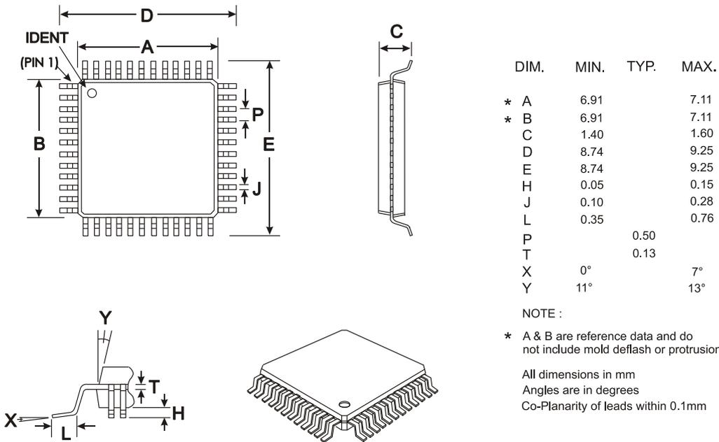
**Figure 27 Mechanical Outline of 48-pin LQFP (L4)**
