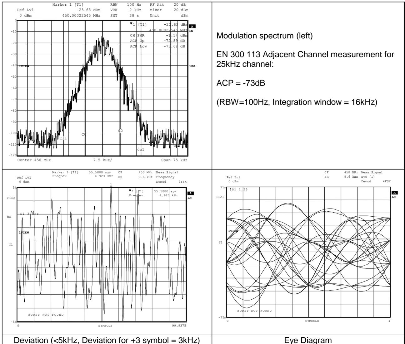
Figure 19 Tx Modulation Spectra (4FSK), 19200bps, 2-point modulation
