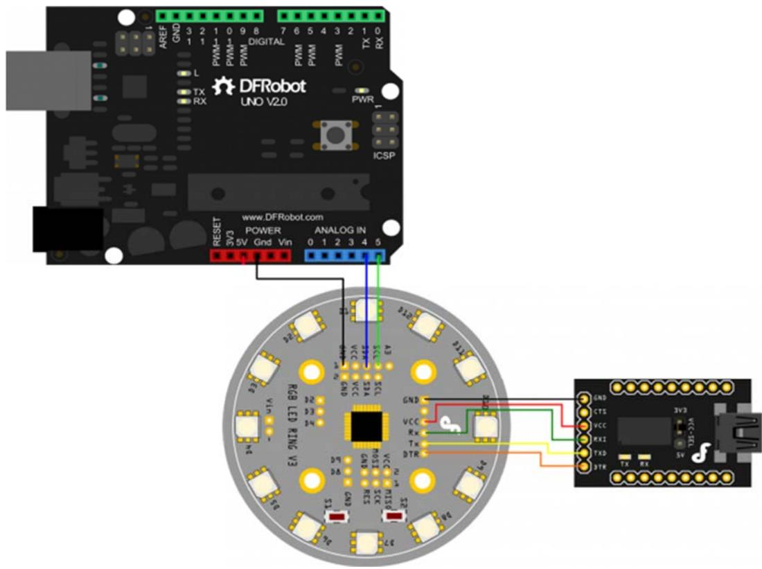
The connection is completed. Then, the UNO as the sender, the *SenderV3.pde* sketch in the folder needs to be uploaded to the UNO, and, the Rainbow Ring as the receiver, the *ReceiverV3.pde* sketch in the folder needs to be uploaded to the Rainbow Ring. Now, you can use UNO's serial to control the Rainbow Ring by different commands.
