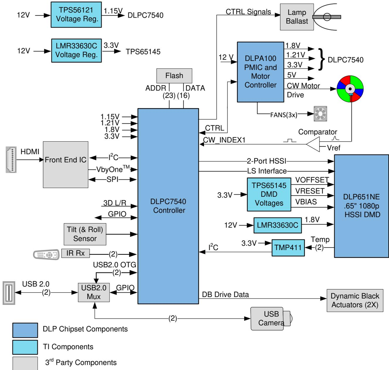
Figure 8-2. Typical 1080p Lamp Phosphor Application Diagram
