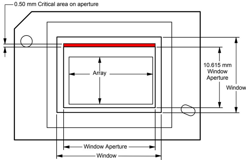
**Figure 6-2. Illumination Overfill Diagram - Critical Area**
