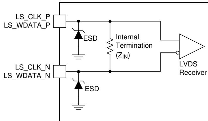
Figure 6-8. LSIF Equivalent Input
