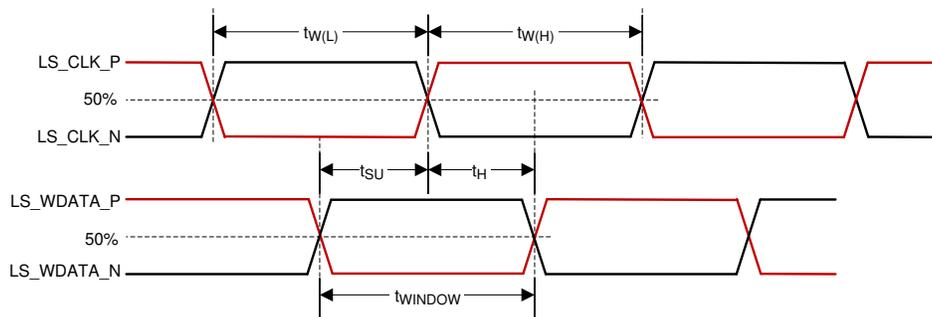
**Figure 6-5. LSIF Timing Requirements**
