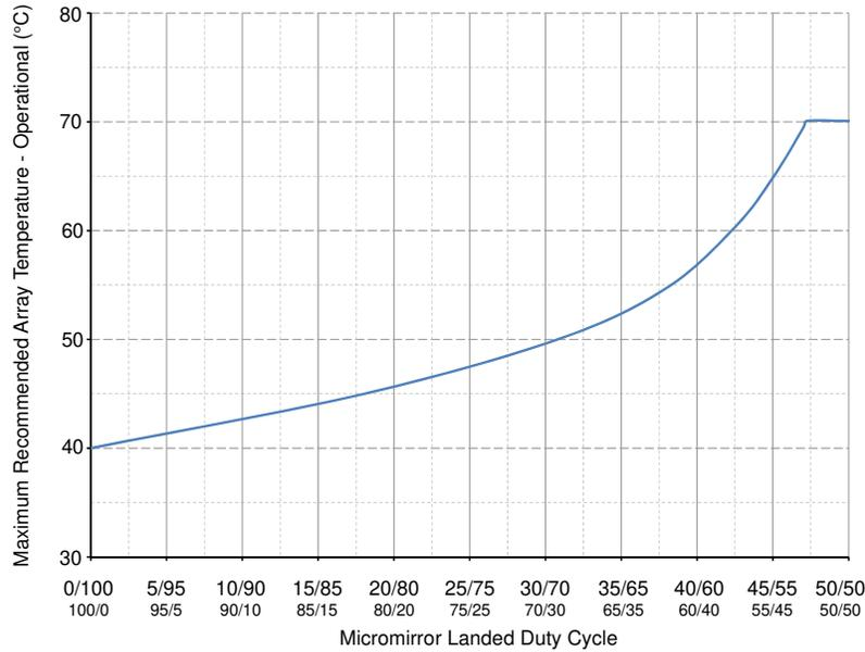
**Figure 6-1. Maximum Recommended Array Temperature - Derating Curve**
