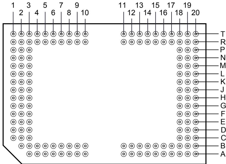
Figure 5-1. FYP Package 149-Pin CPGA Bottom View
