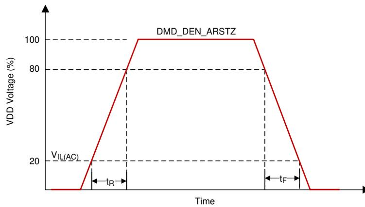
**Figure 6-10. LVC MOS Rise, Fall Time Slew Rate**
