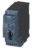
SIRIUS Compact load feeder DOL starter 690 V 24 V AC/DC 50...60 Hz 0.1...0.4 A IP20 Connection main circuit: plug-in, without terminals Connection auxiliary circuit: screw terminal
