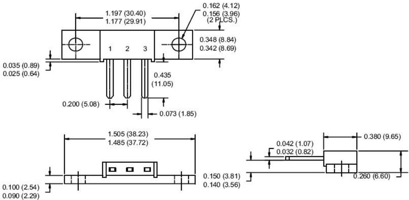
**Mechanical Dimensions PRM2-SL (Inches/Millimeters)**
