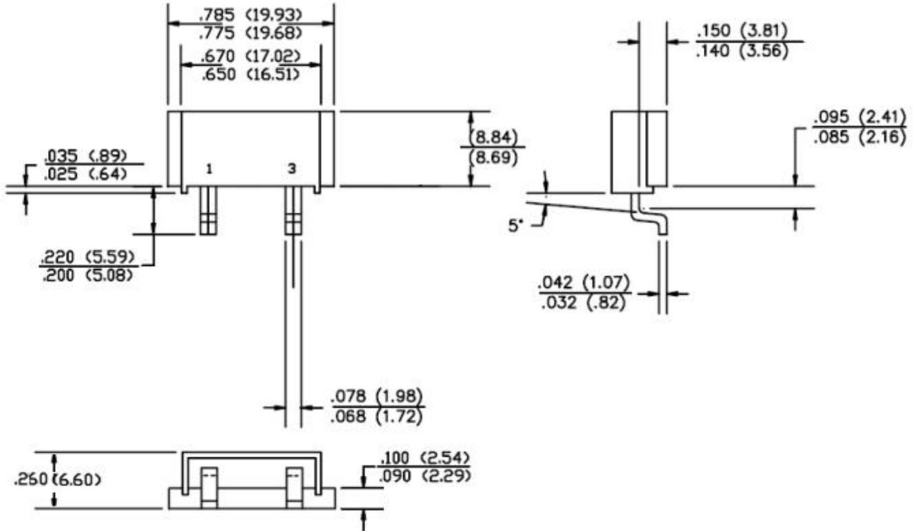
**Mechanical Dimensions PRM2-SM (Inches/Millimeters)**
