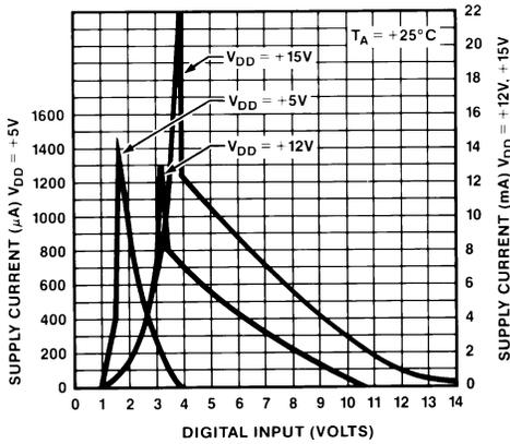
Figure 13. Supply Current vs. Logic Input Voltage
