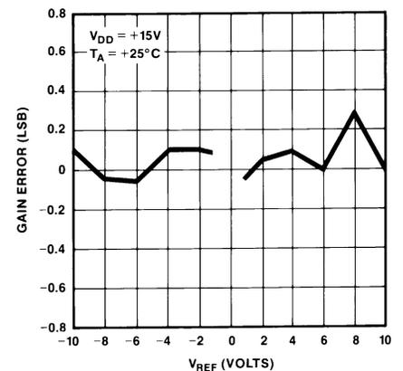
Figure 9. Absolute Gain Error Changes vs.  $V_{REF}$
