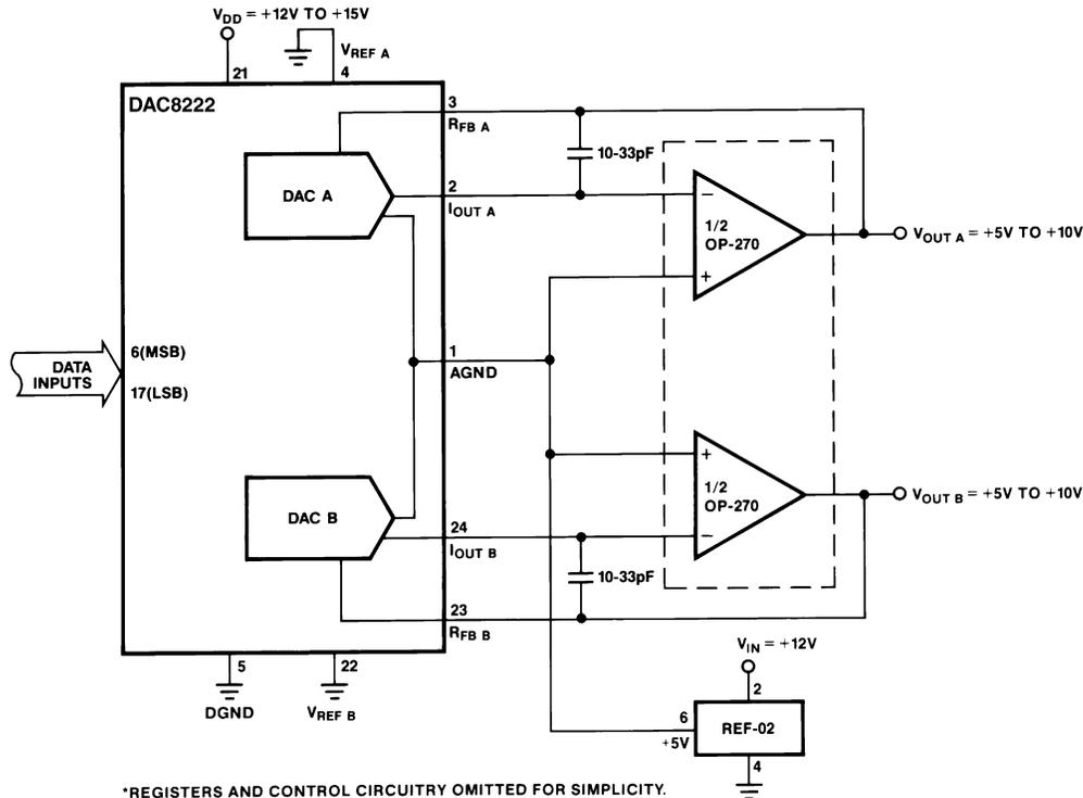
Figure 26. Single Supply Operation (Current Steering Mode)
