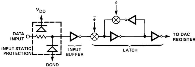
Figure 21. Digital Input Structure For One Bit
