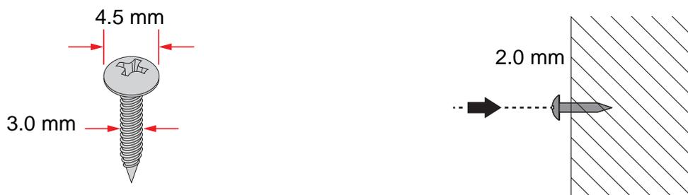
**Figure 2.4 Securing Wall Mounting Screws**
