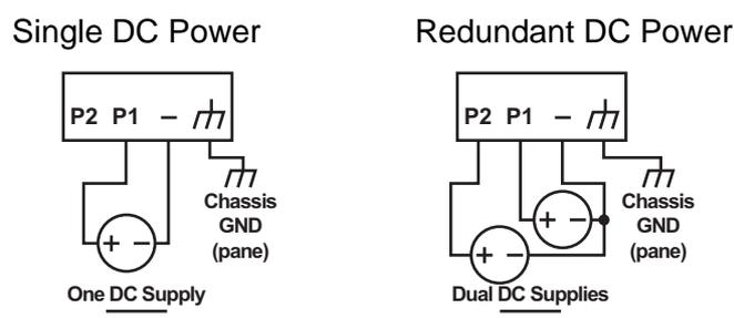
Figure 2.12 Power Wiring for EKI-5500/5600-EI/MB series
