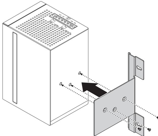
**Figure 2.3 Installing Wall Mount Plates**
