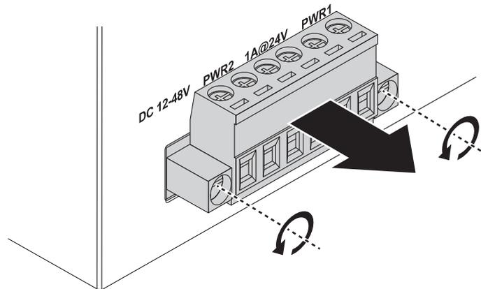
**Figure 2.16 Removing a Terminal Block**
