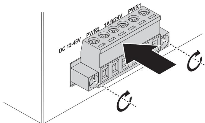
**Figure 2.19 Securing a Terminal Block to a Receptor**
