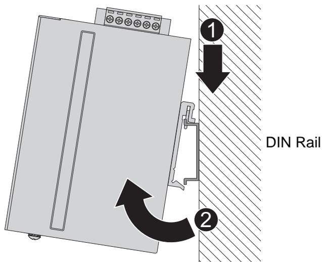
Figure 2.2 Removing the DIN-Rail
