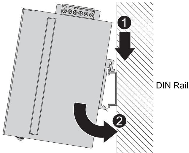
Figure 2.1 Installing the DIN-Rail Mounting Kit
