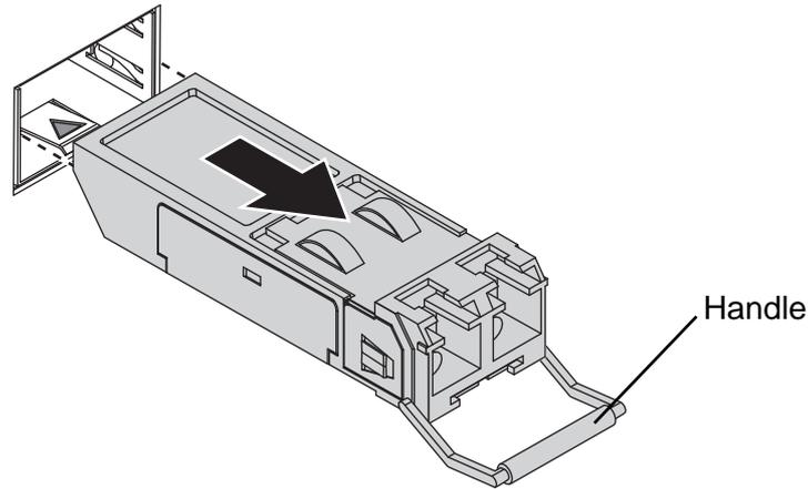
**Figure 2.10 Removing an SFP Transceiver**
