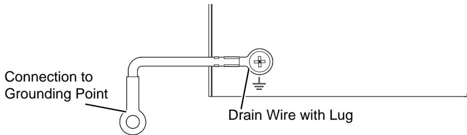
**Figure 2.13 Grounding Connection**
