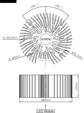
Assembly direction of customer's LED Module
