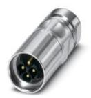
Cable connector, straight, Screw locking, M17, number of positions: 5+3+PE, type of contact: Pin, Crimp connection, shielded: yes, cable diameter range: 8 mm ... 10 mm
