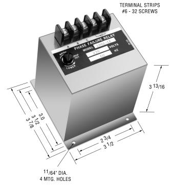
Note: Dimensions in inches. Multiply values by 25.4 for dimensions in mm.
