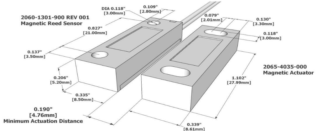
All measurements are in Inches [millimeters]
