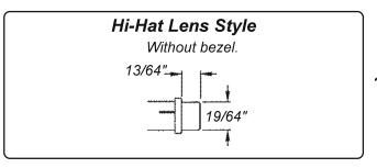
Hi-Hat Lens Variety of Lens Colors 1/8" Tab Terminals or 3/16" Tab Terminals PressFit Mounting
