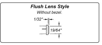
Flush Lens Variety of **Lens Colors** 1/8" Tab Terminals or 3/16" Tab Terminals **PressFit Mounting**
